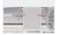
Move centre outlet adjustment lever up, down, left or right by hand to adjust direction of airflow.
