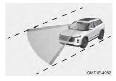
When vehicle speed is no less than 40 mph (65 km/h) and lane line is recognized, LDP enters standby status.
