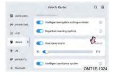
Overspeed alarm function can be turned on or off in the vehicle centre of the audio system.
