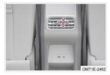
Move rear outlet adjustment lever up, down, left or right by hand to adjust direction of airflow.
