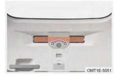
Warning triangle is located on the boot door panel, turn the retaining clamp counterclockwise to remove it.
