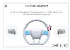
Turn vehicle power to ON mode, Audio System - Vehicle Centre -Vehicle comfort - Rear mirror adjustment.
