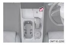
While vehicle power is switched to ON mode, the wireless charging starts to work after putting the mobile phone in wireless charging sensing area, and the audio head unit displays " <sup>(1)</sup>)". The audio head unit displays " <sup>(1)</sup>)" after charging is completely.
