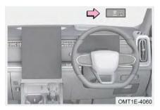
When head up display is turned on, a virtual image is formed in front of driver's field of vision to display the corresponding vehicle speed, driving mileage and other information.
