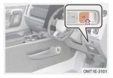
With engine starts or vehicle power is switched to ON mode, depress the brake pedal and press electric parking brake button manually, "(P)" red indicator in instrument cluster and electric parking brake button indicator will turn off, indicating parking brake function has been released.
