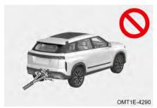
When washing vehicle, use a soft cloth or water (low water pressure) to wash off foreign matter such as snow, mud, and dust on the surface of the radar sensor.
