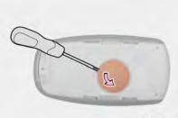
Step 2: Pry off battery cover using a flathead screwdriver with the tip taped, and remove the battery.
