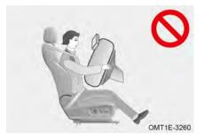
Alwavs keep SRS airbad deployment path clear. It is forbidden to place anything (such as mobile phone) between the occupant and the SRS airbag and fix or place any objects on or near the SRS airbag cover: If there is an object between occupant and SRS airbag, the SRS airbag may not deploy according to design path, or the SRS airbag may push object to occupant's body, causing serious injury or even death.
