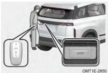
Method 1: With central control lock unlocked, approach the back of vehicle and press exterior switch, on the boot door, directional indicator lights will come on and power boot door will be opened/closed.
