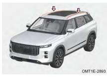
Roof carrier is used to load cargo which can bear 75 kg goods. Overweight will cause carrier, body roof and other components to be damaged, the various problems caused by overweight are not within the claims.
