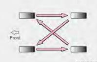
To equalize tyre wear and extend tyre service life, we recommends that you should rotate your tyres approximately every 12 mouths or 10,000 miles (16,093 km); the tyre rotation cycle may vary according to your driving habits and road surface conditions.
