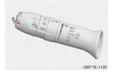
Turn vehicle power to ON mode, pull wiper combination switch towards the steering wheel and hold, the front washer sprays water, and front wiper operates simultaneously. Front washer will stop operating when the switch is released, the wiper will wipe 3 cycles at low speed, and operate one cycle then stop after a few seconds.
