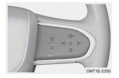
Customization button "  $\overleftrightarrow$  ": This button can be customized in audio system - Vehicle Centre - Vehicle Settings.
