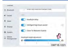
Turn vehicle power to ON mode, headlight height can be adjusted in the vehicle centre of the audio system
