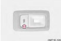
Press rear dome light switch, the light comes on, press the switch again to turn off light.
