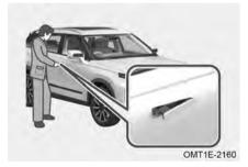
Step 2: Pull the door handle, insert the mechanical key into the keyhole inside the door handle, turn clockwise to unlock the door, counterclockwise to lock the door.
