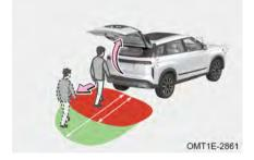
While vehicle power is switched to OFF mode or vehicle is started remotely, four doors are closed, approach to the back (red area) of vehicle when carrying smart key on your person and wait 3 seconds, after directional indicator lights come on, take a step back (green area), power boot door opens.
