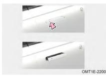
Bring smart key and touch the sensing area of hidden door handle. After system recognizes unlocking signal, the hidden door handle extends automatically, then directional indicator lights flash twice and the door is unlocked.
