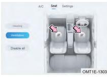
After starting the vehicle, click seat ventilation button by air conditioning display screen - seat - ventilate, it is 3-level ventilation (3 indicators come on). Each time the switch is clicked, the ventilation level is reduced by one level; Click it for the fourth time to turn off the seat ventilation.
