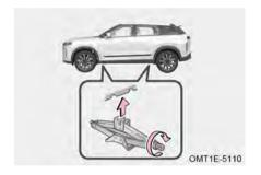
Step 3: Place jack on firm and level ground, turn jack handle clockwise by hand, making the notch of jack contact with the correct jacking-up point.
