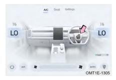
After starting the vehicle, press """ on the air conditioning system screen to turn on steering wheel heating function, press again or work for about 25 minutes, steering wheelheating function is turned off.
