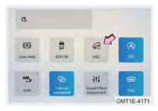
With vehicle power in ON mode, slide down from the top right edge of the audio system screen to display the shortcut menu screen.
