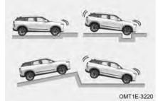
The driver airbag, front passenger airbag, front side airbags, curtain shield airbags and front middle airbag may also deploy if a serious impact occurs to the underside of your vehicle.
