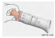
Turn vehicle power to ON mode and operate wiper combination switch.
