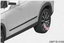
Step 2: Fit wheel bolt wrench to wheel bolt of flat tyre, set the handle on left side, hold the end of wrench handle and push it downward. loosen each bolt of flat tyre about one-half turn:
