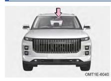
RF emitter and receiver can be placed on back of front windshield for reduced interference etc.
