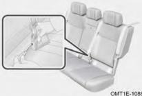
When inserting the small tab into the small buckle of left side of the second row seat. use a screwdriver with its tip wrapped with tape or similar object to press the position shown in illustration and pull out the small tab.
