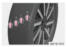
Check the tyre tread by tread wear mark. When tread wear reaches its limit, tread will be in the same plane as the wear band. If such condition occurs, the tyre performance and safety will be seriously impacted, and replacement is necessary.
