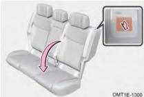
Adjust height of seat head restraints, remove them if necessary and fold up centre armrest. Then pull the left seatback adjustment handle forward and pull seatback forward to fold it down slowly. This can enlarge the luggage storage space.
