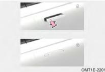
Bring smart key and touch the sensing area of hidden door handle. After system recognizes locking signal, the hidden door handle retracts automatically, then directional indicator lights flash once and the door is locked.
