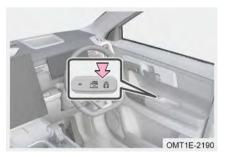
Press passenger side window OFF passenger side window switch. OFF switch indicator comes on. passenger side window switch will be disabled. After disabling, only window switches on driver side can be used to operate passenger side windows (this function is recommended when there is a child in vehicle). Press the switch again to cancel this function and the indicator goes off.
