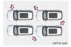
The side airbags, curtain shield airbags and front middle airbag may not deploy if the vehicle is subjected to a collision from side, the rear part of the rear tyre or a side collision at certain angles to the vehicle.
