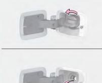
Step 2: Turn fuel filler cap counterclockwise to remove it;
