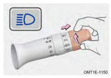
Turn vehicle power to ON mode, when turning on low beam lights, pull headlight combination switch away from steering wheel side and release, high beam lights remain on; Pull headlight combination switch towards steering wheel side and release to turn off high beam lights.
