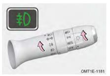
Turn vehicle power to ON mode, when position lights turn on, operate fog light switch to " \$D " position to turn on front fog lights; Turn vehicle power to OFF mode or operate fog light switch to "OFF" position again, front fog lights turn off.
