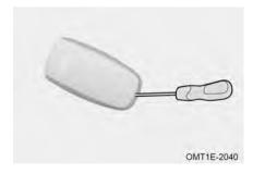
Step 1: Pry off smart key cover using a flathead screwdriver or similar tool with the tip taped.
