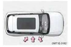
The vehicle is subjected to a strong side impact, and the side collision sensors detect an impact severe enough to cause the side airbags, curtain shield airbags, and front middle airbag to deploy.
