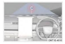
After SLA detects speed limit sign information on road in front and combines the information with speed limit information of navigation system, "<sup>(2)</sup>" indicator in instrument cluster remains on, if the speed exceeds current speed limit, it will have sound prompt or visual warning.
