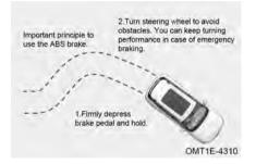
ABS does not function during normal braking and it will be turned on immediately only during sudden braking (brake pedal pulsates with noise, ensuring brake performance and steering performance, if the space is enough, the vehicle can also avoid obstacles). Never release brake pedal in this case.
