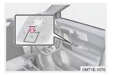
Operate using switch: When vehicle power is turned to ON mode, press outside rear view mirror folding switch to fold mirrors automatically, press the switch again to extend mirrors automatically.
