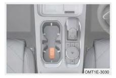
Step 1: Lay smart key onto the key marking of auxiliary fascia console cup holder (as shown in figure) with front side facing up; do not depress brake pedal at this time;
