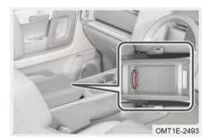
Place necessary items (For example: Canned drinks) in the auxiliary fascia armrest box to perform A/C cooling operation. Rotate inner button of armrest box to cool the necessary items.
