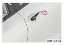
Step 1: Press and hold the front area of the driver door outside handle to open the hidden door handle.
