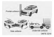
The driver airbag, front passenger airbag and driver knee airbag may not deploy if the front of vehicle hits a telegraph pole, goes under a truck, or if the vehicle is involved in an sideways collision.
