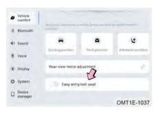
Turn vehicle power to ON mode, turn on easy entry / exit seat function by Audio System - Vehicle Centre -Vehicle comfort.
