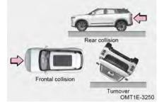
The side airbags, curtain shield airbags and front middle airbag may not deploy if the vehicle is subjected to a front or rear collision, turnover or low speed side collision.
