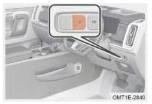
When the power boot door is moving, press this switch to suspend the action.
