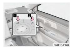
In the vehicle, press lock/unlock switch to lock/unlock the doors.
