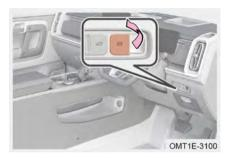
When vehicle power is switched to ON mode, or engine starts and vehicle is stopping, pull up the electric parking brake button, "(<sup>(C)</sup>)" red indicator in instrument cluster and electric parking brake button indicator remains on, indicating parking brake function has been turned on.
