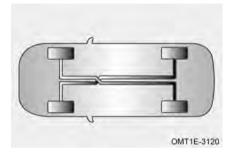
The brake system adopts X type arrangement, double circuit brake system; The system is a hydraulic svstem with two independent subsystems. lf one of the subsystems fails, the other system can still perform brake function. However, the brake pedal should be depressed more firmly than usual and braking distance will the and the brake system increase. malfunction indicator remains on.
