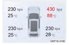
When tyre temperature is higher than 85° C and speed is no less than 15 mph (25 km/h) for a period of time. system will send a high temperature corresponding wheel warning, symbol will blink. current tvre temperature value will be displayed n (!) n and vellow indicator in instrument cluster will remain on.
