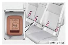
The rear outside seats are equipped with ISOFIX / i-Size anchorages. The anchorage locations are identified by a marking (see illustration) located on the seat back, directly above the associated anchorages. Please press the PUSH position to access the anchorages.
