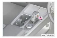
Manual mode: When the transmission gear is in D, press and hold the M switch to enter manual mode M (+, -), push forward to upshift by one gear and push backward to downshift by one gear.
