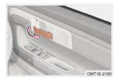
When doors are unlocked, pull door inside handle simply to open door. When doors are locked, pull door inside handle for the first time to unlock the door, and pull it again to open the door.
