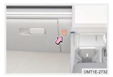
Instrument panel hook is at right of glove box.
