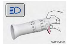
Pull headlight combination switch towards the steering wheel and release it to flash the high beam lights once. At the same time, headlight high beam indicator in instrument cluster flashes once.
