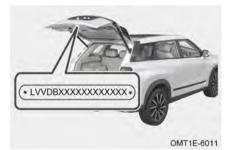
Vehicle Identification Number (VIN) label is located on boot door as shown in the illustration.
