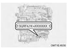
Engine number is located on engine block as shown in the illustration.
