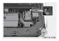
Step 1: Turn vehicle power to OFF mode, and connect jumper cables;
