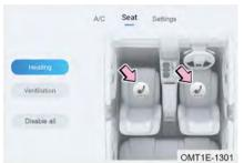
Method 1: After starting the vehicle, click front seat heater button by air conditioning display screen - seat heating, it is 3-level heating (3 indicators on). Each time the switch is clicked, the heating level is lowered one level. Click it the fourth time to turn off the seat heating.
