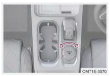
System is ECO mode by default when engine starts. Rotate driving mode knob between SPORT mode, ECO mode or NORMAL mode. You can choose according to different road conditions.
