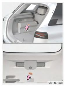
When boot door is opened, luggage compartment lights will turn on for several seconds automatically. When boot door is closed, luggage compartment lights will turn off immediately.
