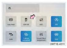
Turn vehicle power supply to ON mode, slide down from the top right edge of the audio system screen, click ESP OFF switch to turn off ESP; click ESP OFF switch again to turn on ESP.
