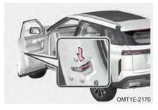
Open the door, move the button downward to lock door; Pull the door handle to make sure the door is locked.
