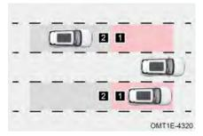
When speed increases to 9 mph (15 km/h) or more, BSD system enters activating; When speed is decreases from more than 9 mph (15 km/h) to 10 mph (10 km/h), BSD system enters pre-activating.
