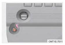
With the engine stalling and cooled down, check the oil level with the dipstick.
