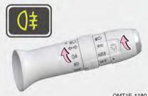
Turn vehicle power to ON mode, when front fog light or low beam lights turn on, operate fog light switch to " O<sup>‡</sup> " position to turn on rear fog light; After turning vehicle power to OFF mode or operate fog light switch to " <sup>()</sup> <sup>‡</sup> " or "OFF" position again, rear fog light turns off.
