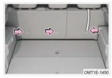
Step 1: Locate the ISOFIX anchorage; Please adjust the second row seat back angle to the front gear.
