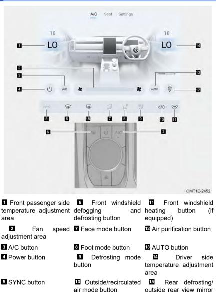
Note: Function buttons are different depending on the vehicle configuration. Please refer to the actual vehicle configuration.
