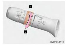
When AUTO mode is selected, the sensor sensitivity can be adjusted by operating the switch.
