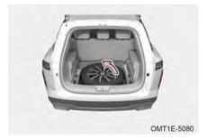
Step 2: Rotate fixing device of spare tyre counterclockwise to remove it, and then take out spare tyre.
