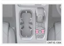
Method 2 (if equipped): After starting the vehicle, press the front seat heater switch on the auxiliary fascia console. it is 3-level heating (3 indicators on). Each time the switch is pressed, the heating level is reduced by one level. Press it the fourth time to turn off the seat heating.
