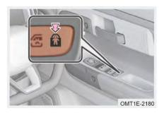
Press the switch, the switch indicator is on, and child-protector lock is locked. At this time, the rear door cannot be opened from inside the vehicle, but only from outside the car.
