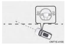
When vehicle speed is no less than 40 mph (65 km/h) and lane line is recognized, LDW enters standby status.
