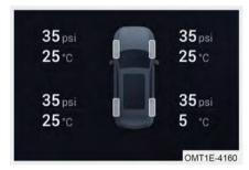
When the driving speed of vehicle is higher than 19 mph (30 km/h) and the continuous driving time is more than 45 s, the instrument cluster can display the tyre pressure and temperature values in real time.
