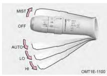
Turn vehicle power to ON mode, move the wiper combination switch:
