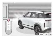
Turn the headlight combination switch to "AUTO" position before stopping. When the vehicle is in a dim environment, press unlock button on smart key, the low beam lights come on for 27 seconds.
