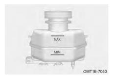
Brake fluid level should be between the "MIN" and "MAX" marks. If the level is at or below the "MIN" mark, add brake fluid and contact the authorized service centre for inspection and repair immediately.
