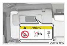
This sticker is attached to front passenger sun visor and used to remind you that the vehicle is equipped with front airbag (SRS). Observe the following precautions:
