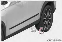
Step 4: When the notch of jack contacts correct jacking-up point, fit jack rocker into jack, and then fit wheel bolt wrench into jack rocker. and turn the wheel bolt wrench clockwise to jack up the vehicle;
