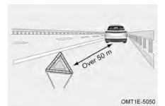
Place the warning triangle at a distance of more than 50 m behind the vehicle on a normal road.
