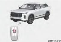
Perform unlocking operation of door to exit locking mode.
