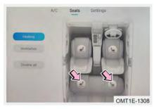
Method 1: After starting the vehicle, click rear seat heater button by air conditioning display screen - seat heating, it is 3-level heating (3 indicators on). Each time the switch is clicked, the heating level is lowered one level. Click it the fourth time to turn off the seat heating.
