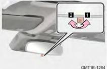
Before driving at night, adjust the inside rear view mirror lever to the anti-glare position, which can reduce the reflected light from the headlights of vehicles behind.
