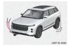
Step 1: Put a block under the tyre diagonally opposite to flat tyre to prevent vehicle from rolling.
