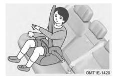
For larger children that cannot fit in a child restraint system with a high back, they may occupy a second row outboard seat using a booster seat. either attached to the lower anchorage points or belted, as described in the instructions provided bv the child restraint system manufacturer.
